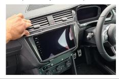
Loosen plastic trimming around the AC controls. Remove 4 x push buttons and set aside AC unit.
