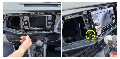
8 Place small bracket in behind and fix into place using provided screw. Use provided self-tapper screw to secure second location.
