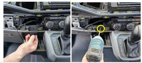
5 Place second bracket behind and use provided screw to fix into place. Then use provided selftapper screw to secure second location.
